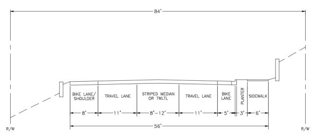
Figure 6 – Three-Lane base design proposed cross section (in Sammamish, facing south)
