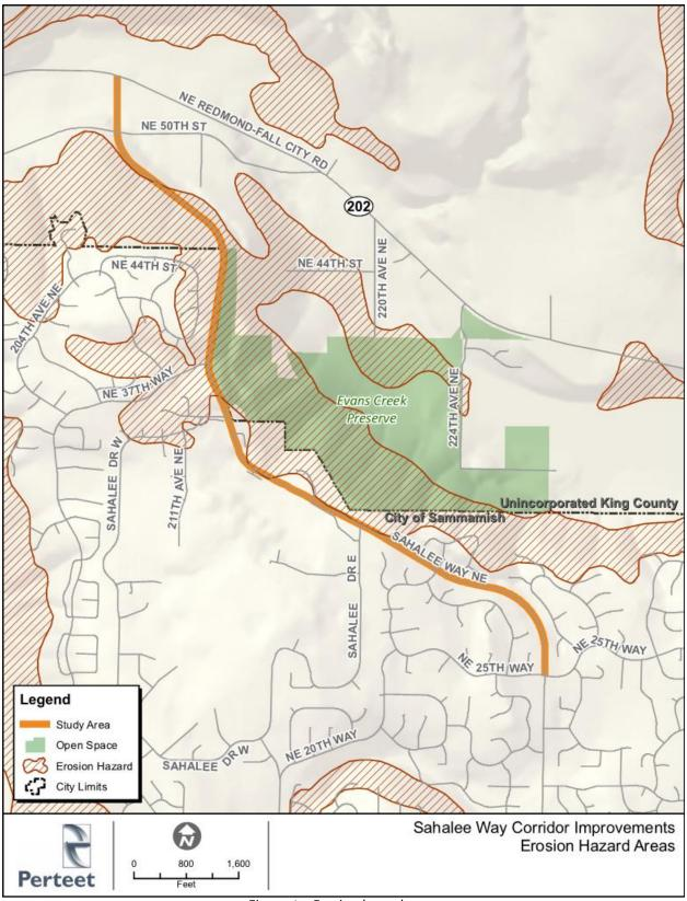
Figure 4 – Erosion hazard zones
