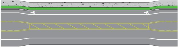
Figure 7 – Narrow median with dual lane re-alignment (not to scale)
