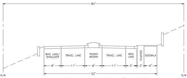
Figure 8 – Raised median island typical section (facing south)
