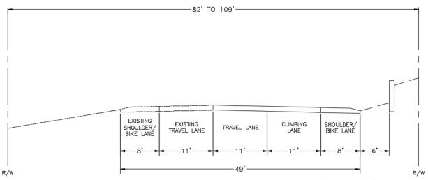
Figure 9 – Three-Lane design with truck climbing lane cross sections (facing south)
