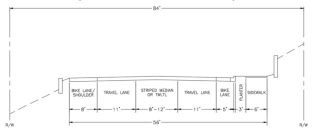
Figure 1 - Three-Lane base design proposed cross section (in Sammamish, facing south)
