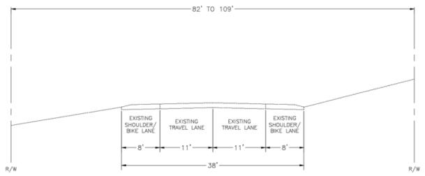
Figure 2 - Existing cross section North of NE 37th and in King County
