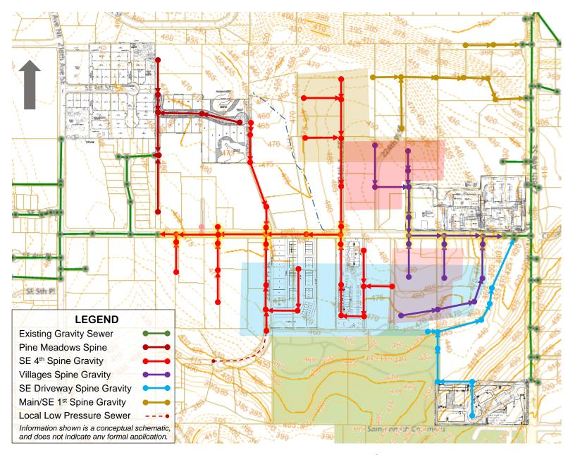
Highlighted lines indicate sewer mains currently proposed for construction
