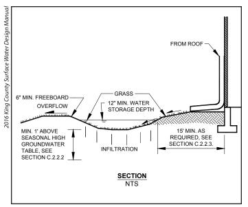
Typical ground surface depression infiltration system.
