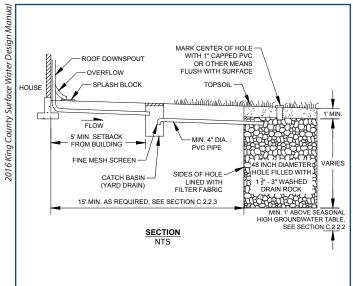
Typical drywell infiltration system.
