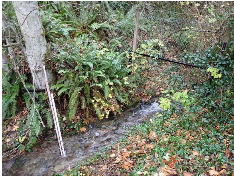
Photo 3 Lower George Davis Creek stage recorder inside PVC stilling well
