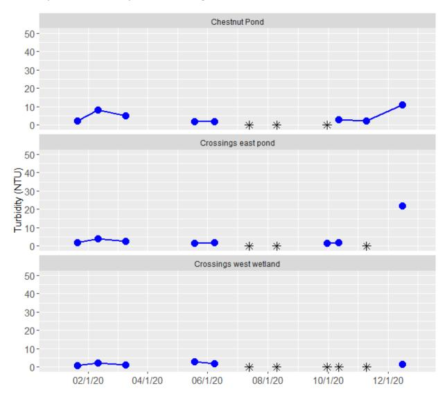
Blue dots show turbidity values, and black asterisks at zero turbidity indicate dates when the outfall was dry.
