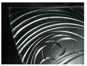
The glass is fired up to 1600 degrees and then cooled and annealed for several days for strength. The slab is 2 inches thick and weighs 400 pounds.
