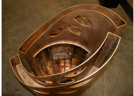
The 1/4" bronze is cut, mill rolled into the radius of the glass and welded. Greg Lundgren and Chris Flechtner of Gulassa take measurements to insure a good fit. Gulassa sets the light and applies the final patina to the bronze.
