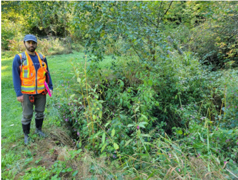
Photo 26. Thickly vegetated and incised channel (right) near the downstream limit of the upper residential reach, facing upstream, near STA 2260. Note, NHC personnel standing adjacent to scarp at slumped bank (September 2023).
